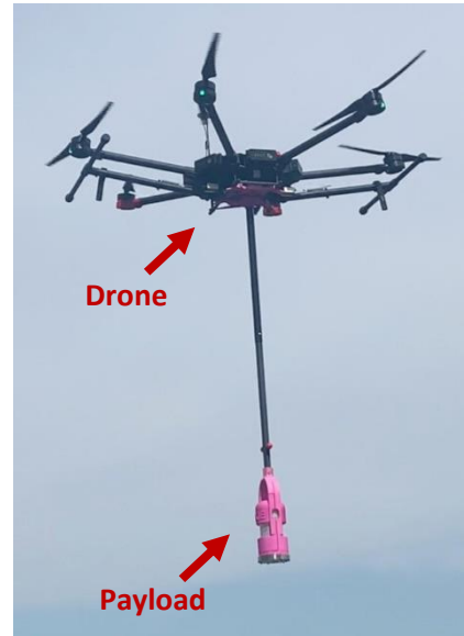
Figure 1. Drone outfitted with water collection payload 1
